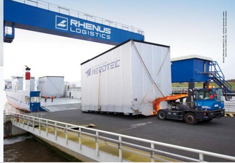
The Blexen terminal has a bridge crane with a carrying capacity of up to 21 tonnes and a hydraulic RoRo pier for loading of various large components.
